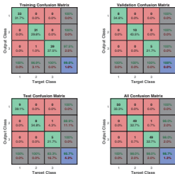
Figure 6.9 Summary of the error performance through confusion matrices of the NN architecture for training, validation and test sets. This figure is accessed with the confusion button on the NN interactive tool of Fig. 6.6.
