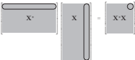
Figure 1.7 Correlation matrix X^*X is formed by taking the inner product of columns of X .
